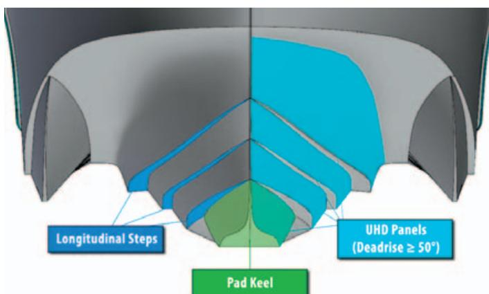
The anatomy of a Sea Blade hull – narrow main hull made of steep risers and small flats that run full length, with an ama each side to form a tunnel and add stability.
