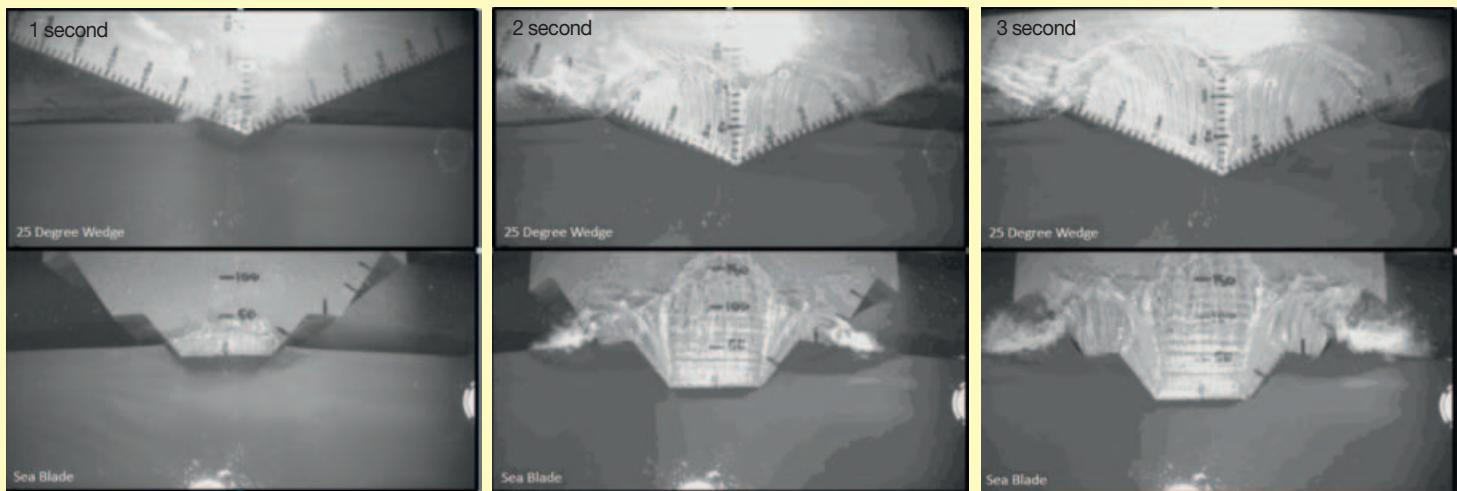
Three image sequence showing how the Sea Blade hull breaks the fall with the flat keel pad and then the smaller flat steps with 50-degree vee between them compared to a 25-degree deadrise vee bottom at 0.01 seconds, 0.02 seconds and 0.03 seconds after impact.
