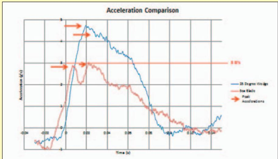
This graph shows the peak slamming pressures of a 25-degree, deep vee hull compared to a Sea Blade hull. The Sea Blade hull has two small peaks at around 3G's spread out over time, while the conventional hull has one big 5G peak over a shorter period. Lower G loads over a longer time are more comfortable for the occupants.
